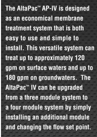
The AltaPac™ systems are fully functional, self contained skids which have all of the features and benefits of the full scale AltaFilter™ including automated operation and daily integrity tests.
