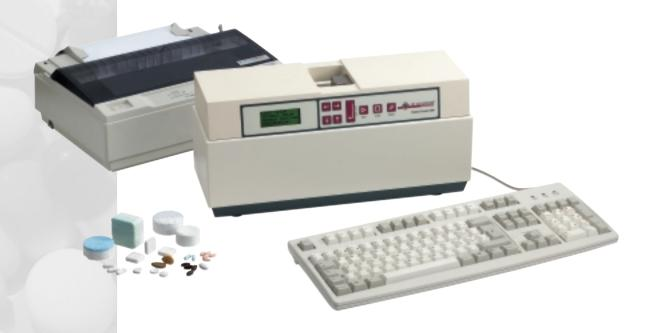
The tablets are inserted manually, one after the other, into the unit. Sample shapes and forms, which cannot be accommodated by automatic machines, are ideally suited for testing with the 8M.
