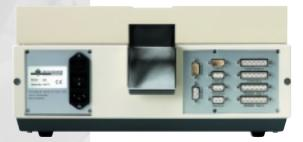
The functionality of the 8M can be extended by attaching an external thickness gauge and analytical balance. In addition, the tester has connections for an external keyboard and printer. The system can be integrated with other devices and data collection systems via an RS232C or CAN-bus interface.
