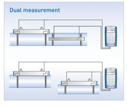
Determination of heat flow volume using the measured volume flow and the difference between the inlet and outlet temperatures.
