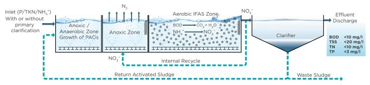
Note: Adding a post-denitrification step can reduce total nitrogen even lower, to < 3 mg/l. TSS removal can be enhanced by further filtration.
