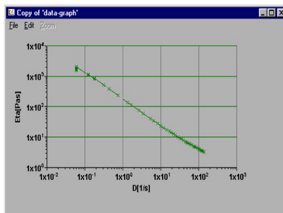
Figure 3: Viscosity Flow Curve Using Controlled Rate Test Method
