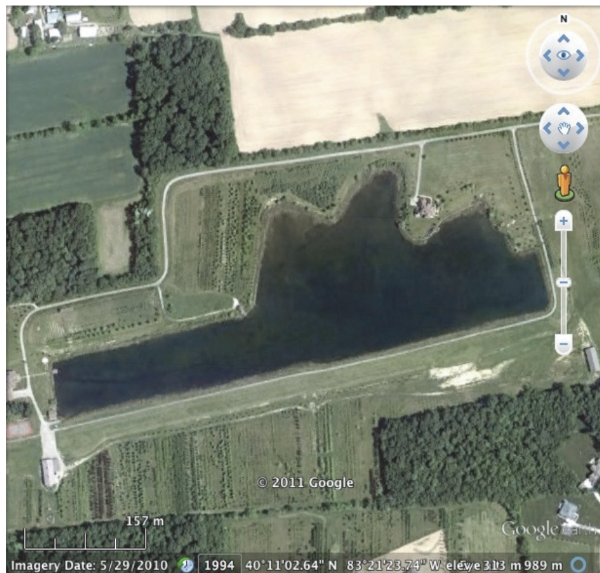
Figure 1 – An Ohio facultative lagoon that is short circuited at its western inlet and it has developed sludge buildup on all its northern banks, as well as most of its other banks.
