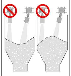
**Liquids Installation Recommendations**Avoid installations where vessel obstructions or fill lines interfere with beam path.
