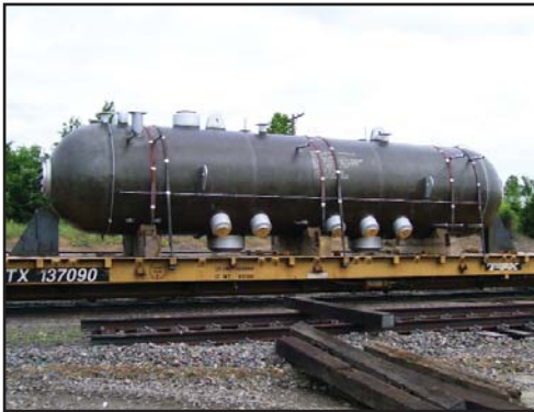
Pressure Vessels (Steam Drum)
