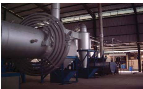
Activation kiln with waste heat boiler
