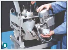
Replace components, reposition motor and drive assembly, tighten quill nut, replace backplate and you're ready to run – all in under two minutes.
