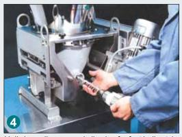
Helix is easily removed allowing for fast helix style and diameter changes.
