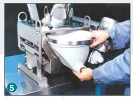
Release band clamp for easy hopper removal. Hopper simply slides out for cleaning, replacement, or maintenance.
