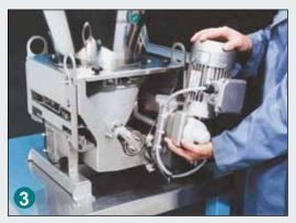
Motor and drive assembly swings back for complete access to all internal components for easy cleaning, reconfiguration, or maintenance.
