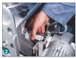
Loosen swivel stop bolt and quill nut.
