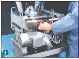
All components are accessible from the rear of the feeder instead of the discharge side. Simply loosen screw knobs and remove backplate.
