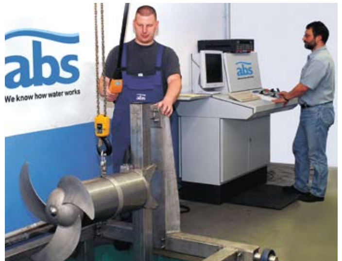
Thrust measurement facility regarding ISO 21630.
