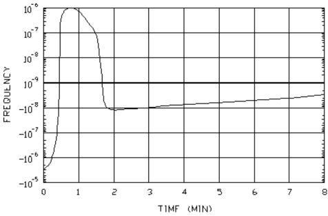
Stabilization Time (warm-up) for an OCXO is defined as the time taken to reach a certain level of stability after a long period of inoperation. Oven power decreases with time during warm-up, reaching a steady state when the oven has reached its operating temperature.
