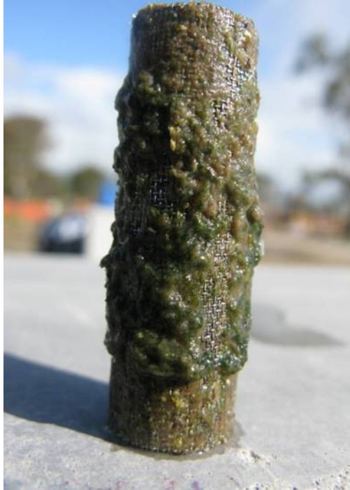
Example of a plugged screen, resulting in an ACV failure
