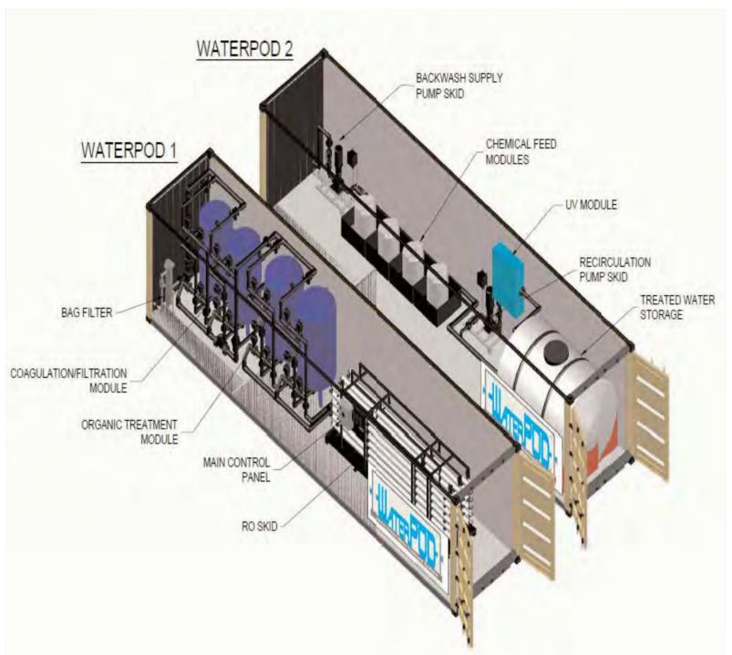
AdEdge WaterPod systems remove a variety of contaminants including arsenic, iron & manganese, uranium, radium, nitrates and TDS among others. The WaterPod systems can be customized to your treatment needs in a variety of configurations and treatment solutions.
