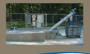
The CLT Series is designed for primary screening of effluents flowing in open channels. They use a shaftless screw to transport, wash, and compact solids that have been captured on a fixed submerged screen element. The CLT – A model adds an agitator device to break up soft organic solids.
